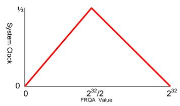
For values of FRQA which are not a power of 2, ( $FRQA \neq 2^N$ ) there will be jitter present on the output signal since the most significant bit of PHSA will toggle at an inconstant rate.
