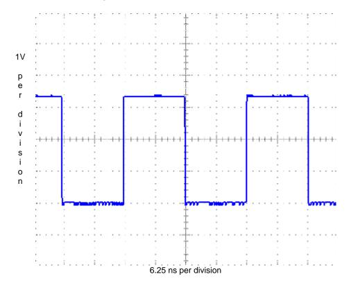
If the mode were changed to %00101 (NCO differential) the output would appear as Figure 4: the blue (dark) line is APIN output signal and the red (light) line is BPIN output signal.
