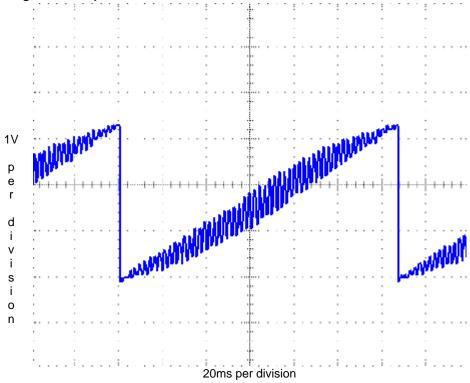
The jaggedness of the saw tooth is due to the switching of the signal and can be smoothed with the addition of a resistor and capacitor to the output.
