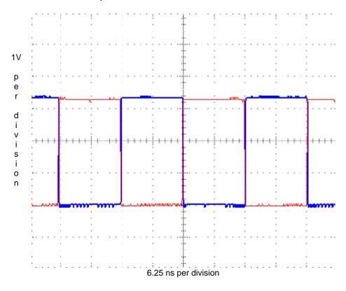
If the master clock is running at 80 MHz, the resultant output on APIN will be 40 MHz or  $\frac{1}{2}$  the system clock. If the contents of FRQA were changed to \$4000\_0000, the sequence of PHSA would be \$0000\_0000, \$4000\_0000, \$8000\_0000, \$C000\_0000, \$0000\_0000,... This would result in PHSA[31] to have the sequence 0,0,1,1,0,... or  $\frac{1}{4}$  the system clock.
