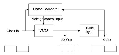
The PLL shown in Figure 7 doubles the input clock frequency and provides two frequencies as output, the input frequency and twice the input frequency. The PLL located in each counter multiplies the input frequency by 16 and provides 8 output frequencies (16x, 8x, 4x, 2x, 1x, 1/2x, 1/4x and 1/6x the input frequency).
