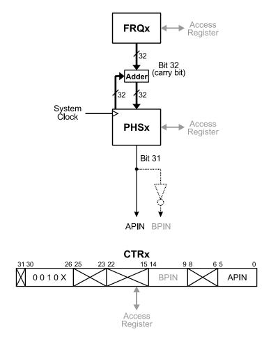
For example, if the APIN is set to 0, the mode is set to %00100 (NCO single-ended) and FRQA is set to \$8000\_0000 as in the following code.
