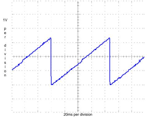
The voltage presented at Out of the circuit is  $(3.3 \times x)/period$  due to scaling the input value by \$20C49B.
