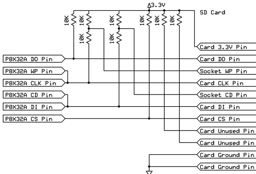
**Figure 4: Micro SD Card Slot Advanced Interface**
