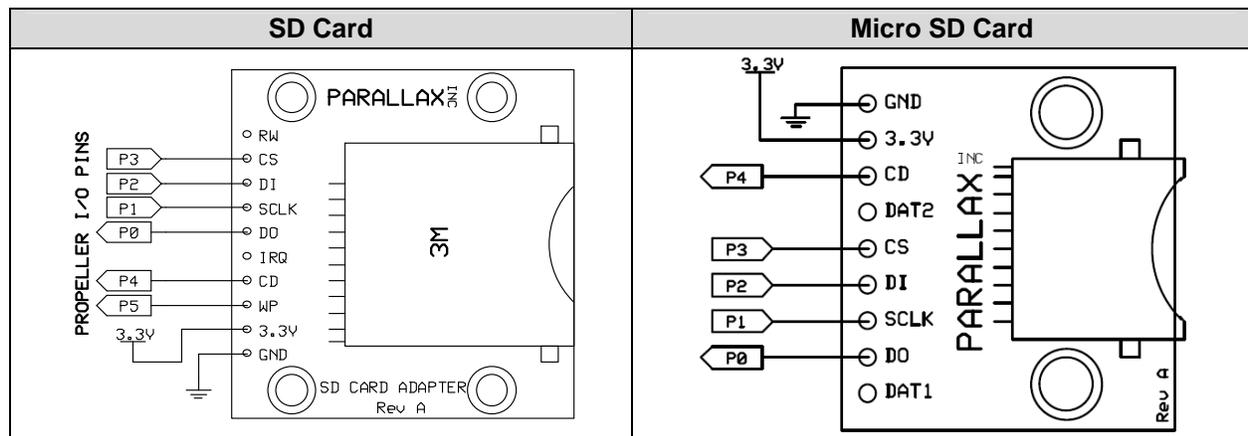
P0 connects to the driver's DO pin, P1 connects to the driver's CLK pin. P2 connects to the driver's DI pin, P3 connects to the driver's CS pin, P4 connects to the driver's CD pin, and P5 (if present) connects to the driver's WP pin. Other pins on the Propeller chip than the ones listed above will work with the Full File System Driver.
