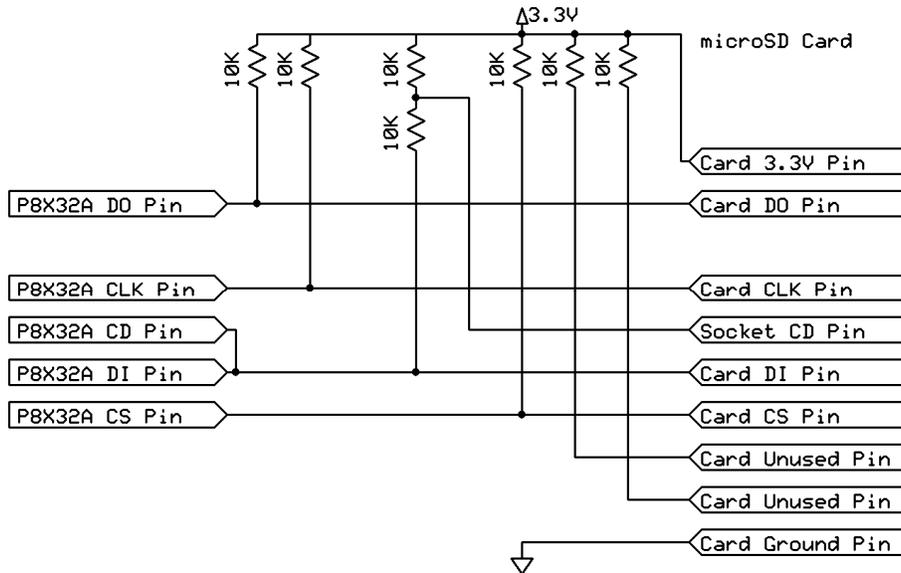
Additionally, connect a power supply decoupling capacitor (above 100  $\mu$ F) and/or filter (not shown above) near the SD or micro SD card slot to prevent brownouts from occurring.
