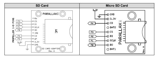
PO connects to the driver's DO pin, P1 connects to the driver's CLK pin. P2 connects to the driver's DI pin, P3 connects to the driver's CS pin, P4 connects to the driver's CD pin, and P5 (if present) connects to the driver's WP pin. Other pins on the Propeller chip than the ones listed above will work with the Full File System Driver.
